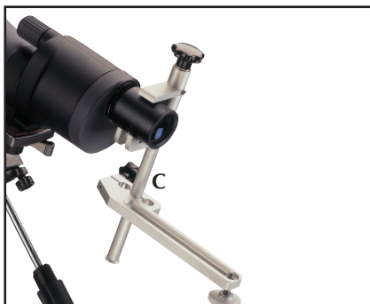
[Fig. 2] Fixing the Balance Plate Assembly
